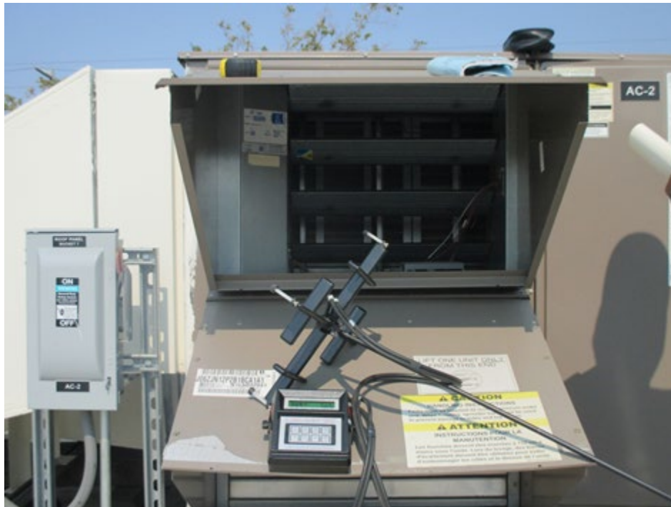
FIGURE 7: TYPICAL FIELD TEMPERATURE MEASUREMENTS – SPUR (LEFT) AND IR GUN (RIGHT)
