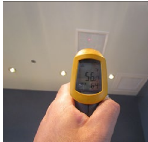
FIGURE 7: TYPICAL FIELD TEMPERATURE MEASUREMENTS – SPUR (LEFT) AND IR GUN (RIGHT)
