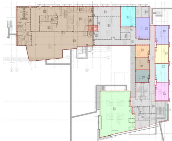
FIGURE 12: EXAMPLE FLOOR PLAN OF DOAS VENTILATION ZONES WITH MANY DCV ZONES, DAVIS SITE
